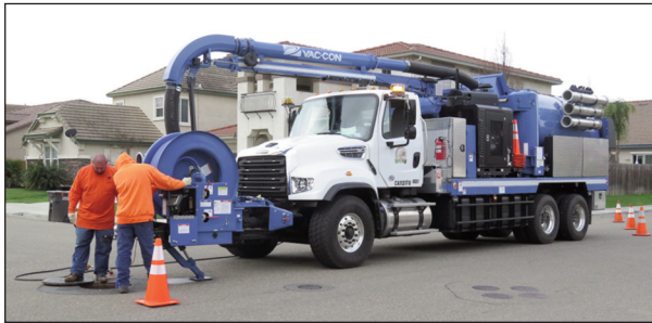
ISD's new Vac-Con sewer-cleaning truck has been on the job since winter. It is larger and more powerful than the vehicle it replaces.
