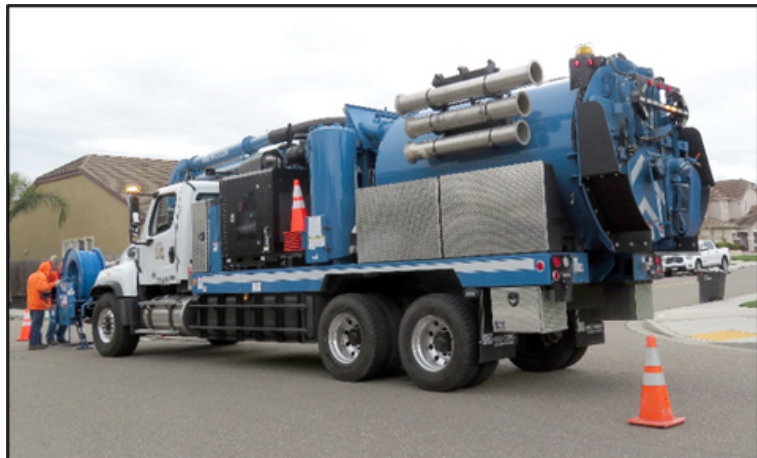
Collections staff prepare to utilize a sewer jet/vacuum truck.
