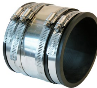
Fernco® Stainless Steel Shear Rings (60 in-lb)
